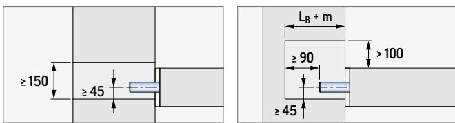
Picture 37 Preparing the precast element for installation
